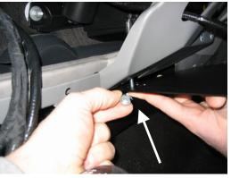
Attach lower portion of console using 1/4" x 1 1/4" hex bolt, washer and serrated nut
